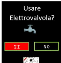
When the Manual mode is set you can also choose to use or not the drain valve. If you set "SI" the key "stop/menu" is activated in order to stop the shot and discharge the residual pressure.
