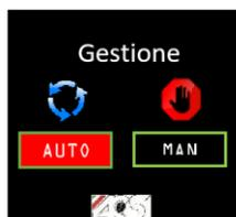
In the first page in setting mode you can choose between Automatic or Manual working. In the Automatic function you can decide later to work by time or pressure while in Manual mode the system is disabled and only the “Stop” button works to stop the shot or in any case to discharge the pressure from the group.
