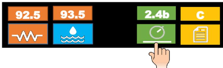
By pressing the pre-infusione key you can set the pressure between 1 and 6 bars.
