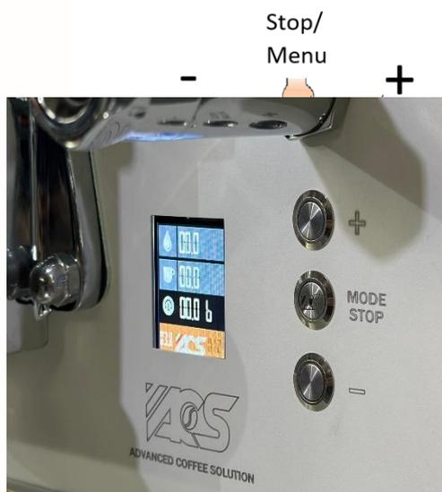
The keys – and + are used to increase and decrease the values during the programming and also move between the different functions. When we are in the main screen the keys up and down are used to choose between the 2 settings available.
