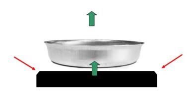
the green arrow and then the entire assembly pushes into the E61 group. The red arrows show the correct orientation of the black gasket, which should be with the angled (chamfered) edge uppermost.
