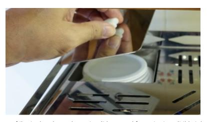
valve" vent tube and need not reach the base of the tank or be under water. It is normal for water to exit this tube during an espresso shot, when the machine is heating after a shot, or on initial warm up. Make sure both tubes are in the tank and not kinked, **do not place the inner lid on the tank, or replace the tank cover at this time.**
